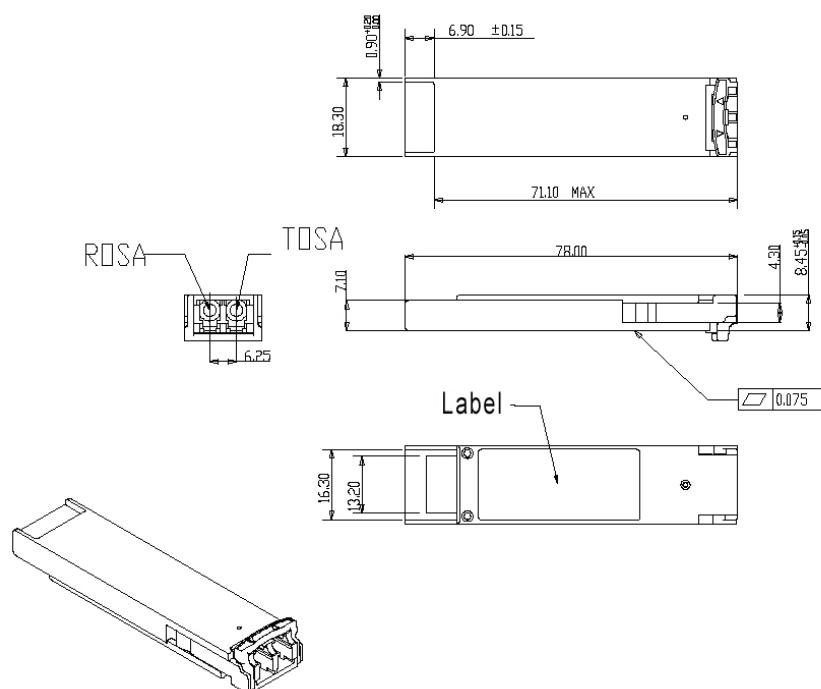
**Figure3. Mechanical Specifications**
